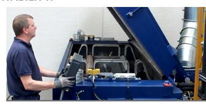
removable washing basket, and then pushed into a front-loaded machine with a closed washing chamber and separate cleaning solution tank. A removable strainer ensures that any loose debris or parts cannot damage or disable the machine or components, and the automatic solvent control system minimizes solvent vapors and regulates solvent concentration. 5 cycles - wash, drain, rinse, secondary drain, air extraction - can each be selected individually based on the needs of the parts to be washed.
